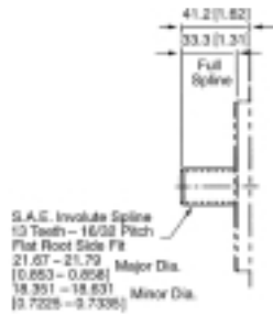
SAE "B" SPLINE (CODE 65)
