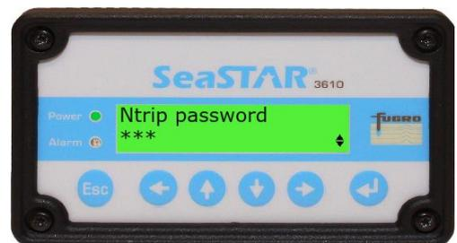
Reboot (restart) the demodulator by holding down **ESC** and **ENTER** at the same time. When the device has rebooted NTRIP will be enabled.
