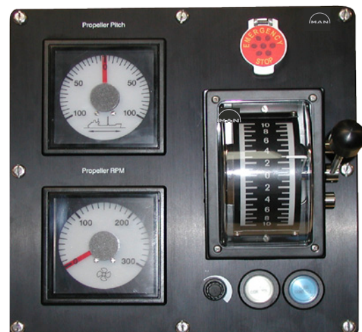
Fig. 11: Bridge manoeuvre panel – bridge wing outdoor
