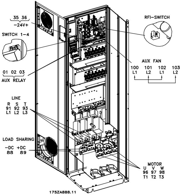
**IP 54, IP 21/NEMA 1 with disconnect and main fuse**
