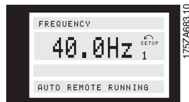
Line 2 gives the current output frequency and the active Setup.
