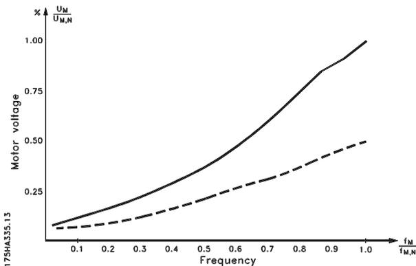
If the AEO function has been selected in parameter 101, *Torque characteristics*, this function will be constantly active. If there is a major deviation from the optimum U/f ratio, the frequency converter will quickly adjust itself.
