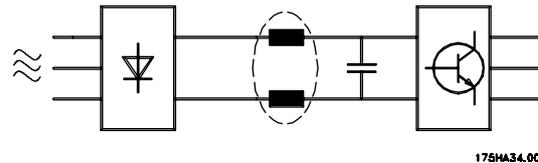
The voltage distortion on the mains supply depends on the size of the harmonic currents multiplied by the mains impedance for the frequency in question. The total voltage distortion THD is calculated on the basis of the individual voltage harmonics using the following formula:
