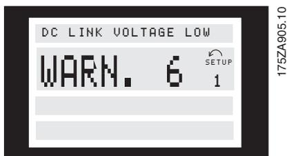
If an alarm is given, the present alarm number will be shown in line 2. Lines 3 and 4 of the display will offer an explanation.
