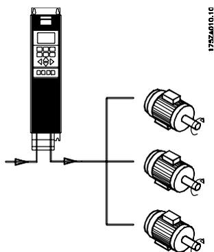
VLT 6000 HVAC is able to control several motors connected in parallel. If the motors are to have different rpm values, the motors must have different rated rpm values. Motor rpm is changed simultaneously, which means that the ratio between the rated rpm values is maintained across the range. The total current consumption of the motors is not to exceed the maximum rated output current  $I_{VLT,N}$  for the frequency converter.
