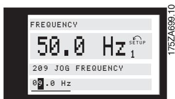
Then the chosen digit is changed infinitely by means of the [+/-] keys:
