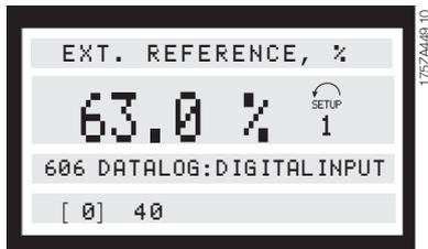
Data logs [1]-[20] can be read by first pressing [CHANGE DATA], followed by the [+/-] keys to change data log numbers.
