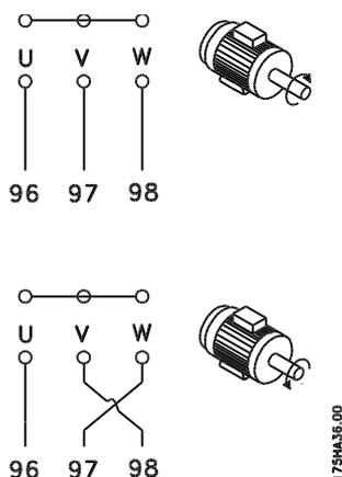
The factory setting is for clockwise rotation with the frequency transformer output connected as follows.
