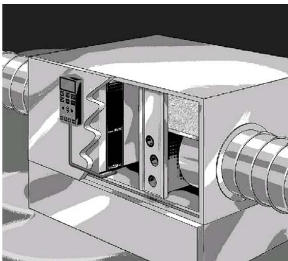
This example shows an application with *Run permissive*, warning against no load and warning for filter change.
