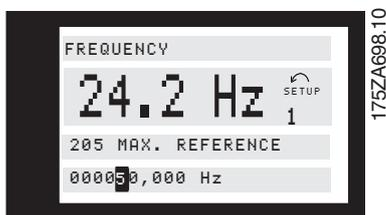
The selected digit is indicated by a flashing cursor. The bottom display line gives the data value that will be entered (saved) when signing off by pressing the [OK] button. Use [CANCEL] to cancel the change.
