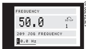
The chosen digit flashes. The bottom display line shows the data value that will be entered (saved) when signing off with [OK].
