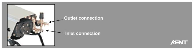
Connect the water supply to the cold-water cleaner by a 3/4 inch. fabric-reinforced hose. Use tap water or "reject water" (treated waste water), if available.
