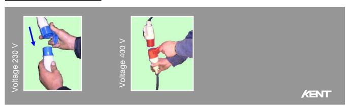
Any repair or adjustment must take place only when the main power has been locked and the highpressure cleaner has been secured against accidental start-up. A removable power plug makes the technician even safer.
