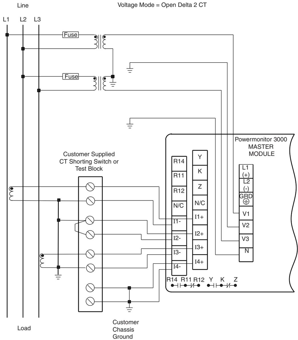
**Figure 24 3-Phase 3-Wire Grounded L2(B) Phase Open Delta Direct Connect with Three CT's Wiring Diagram(Systems ≤ 600 Volts Nominal L-L)**
