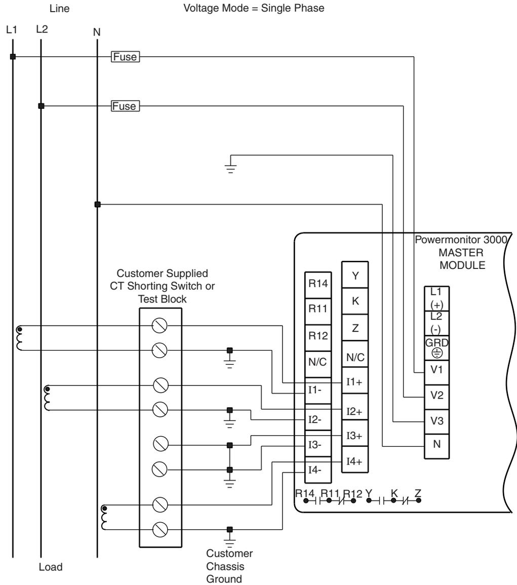
**Figure 15 Single Phase with PTs Wiring Diagram**
