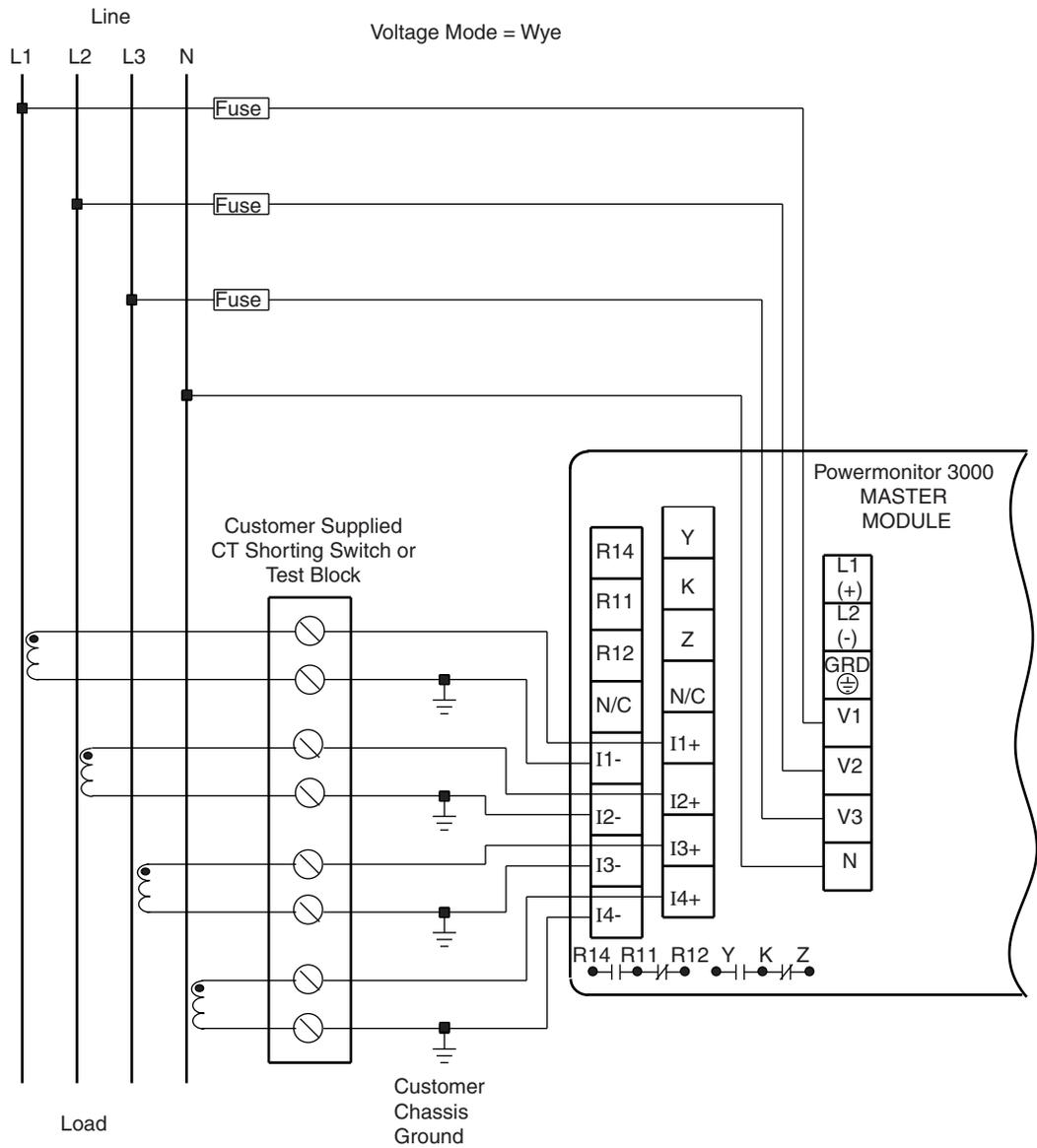
Figure 17 3-Phase 4-Wire with PT's Wiring Diagram
