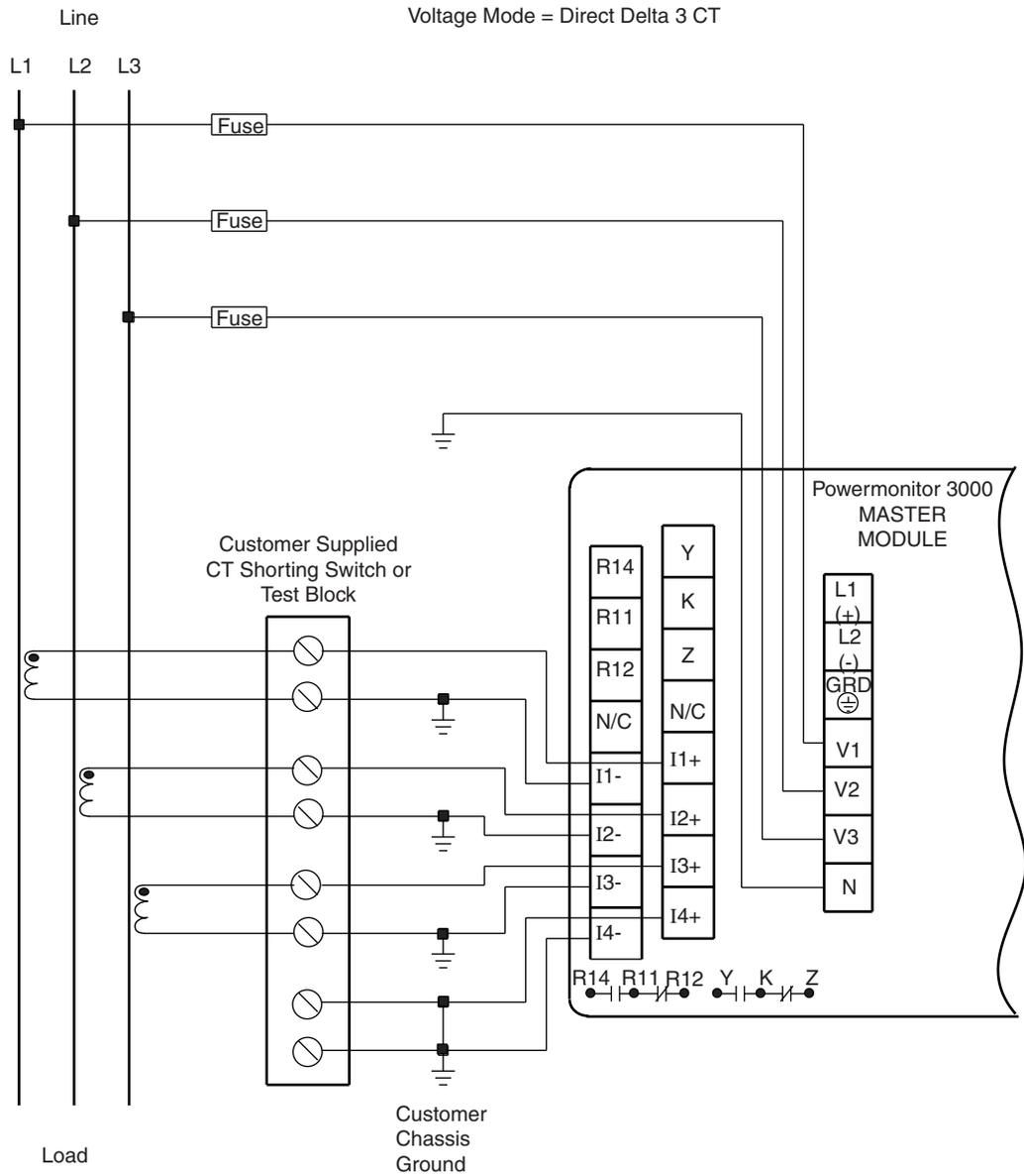
**Figure 26 3-Phase 3-Wire Delta Direct Connect with Two CT's Wiring Diagram
