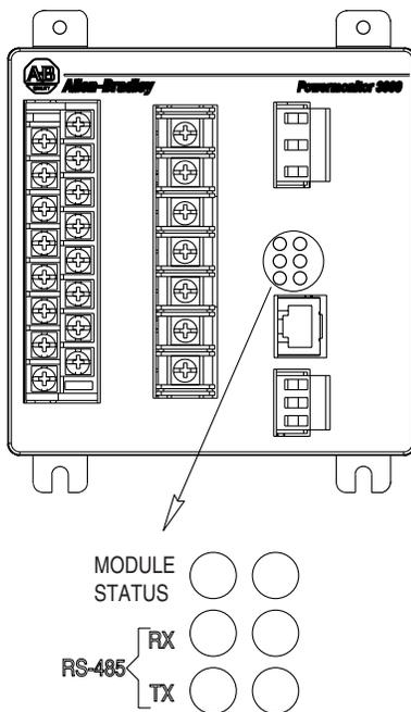
The three LED's on the left display the same information on Powermonitor 3000 modules with any communication option including native RS-485 communications only. The three LED's on the right have different labels and different indications depending on the communications option selected, as shown in the charts below.
