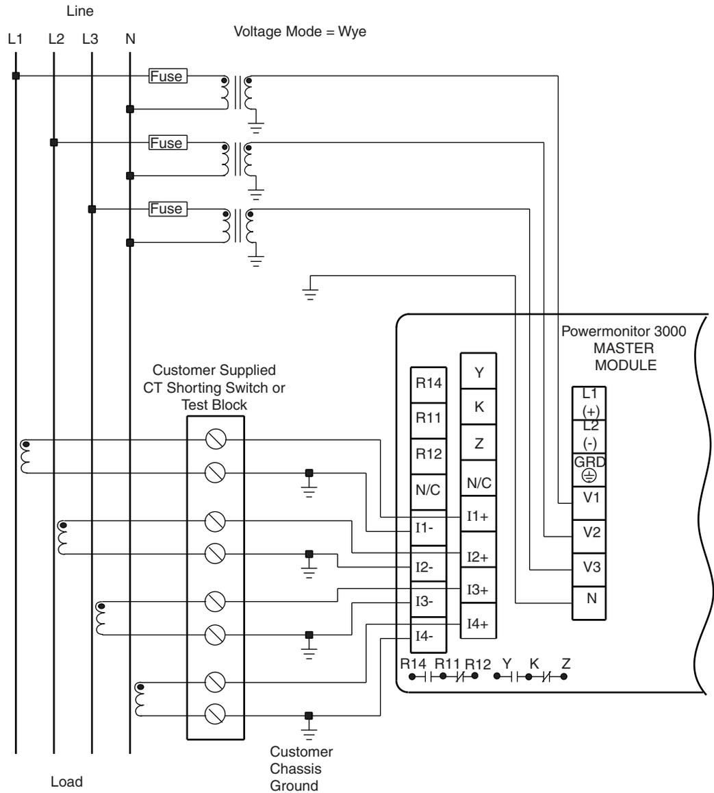
**Figure 18 3-Phase 3-Wire Grounded Wye Direct Connection Wiring Diagram
