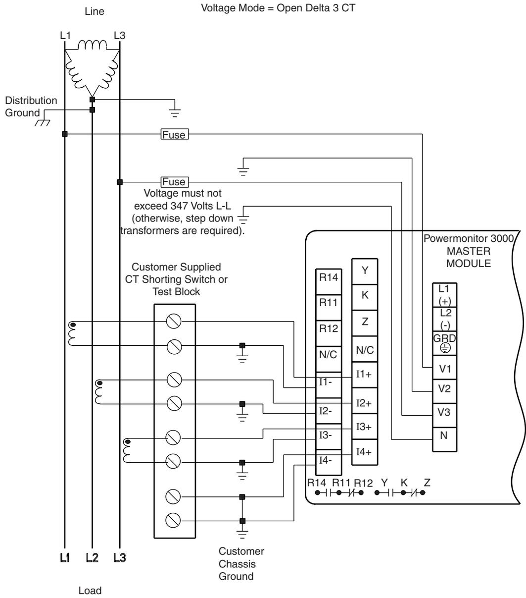
**Figure 25 3-Phase 3-Wire Delta Direct Connect with Three CT's Wiring Diagram
