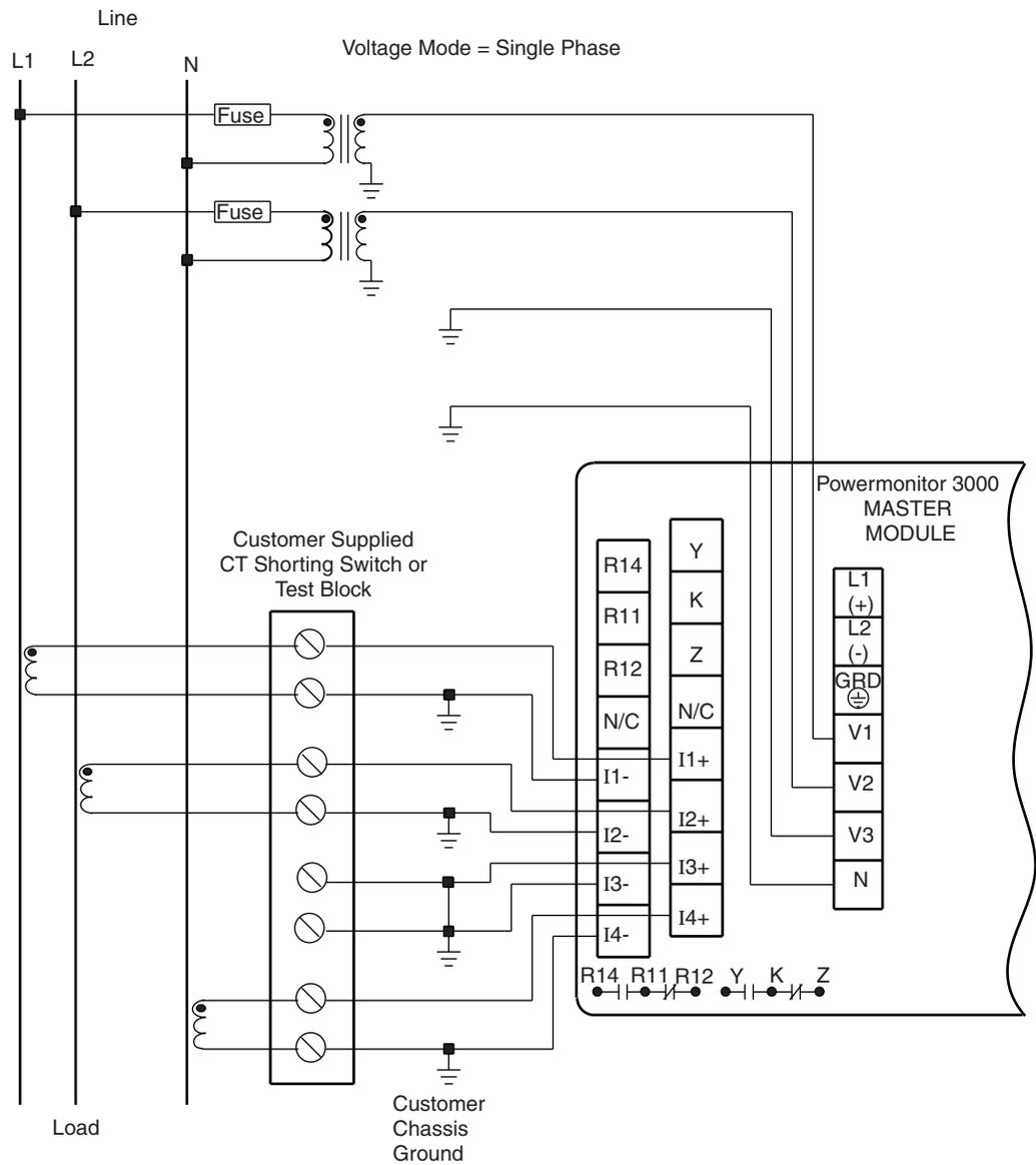
**Figure 16 3-Phase 4-Wire Wye Direct Connect Wiring Diagram
