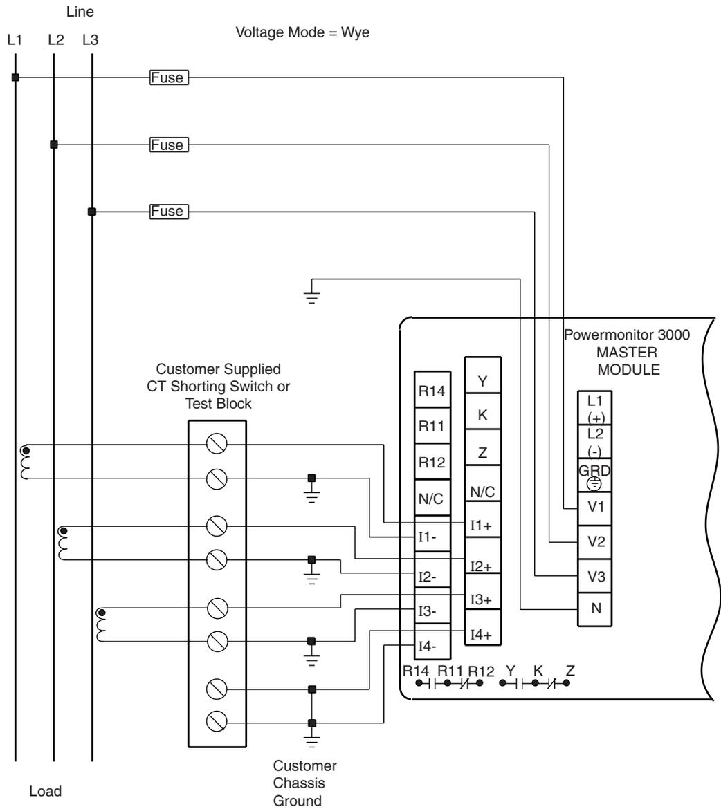
Figure 19 3-Phase 3-Wire Grounded Wye with PT's Wiring Diagram
